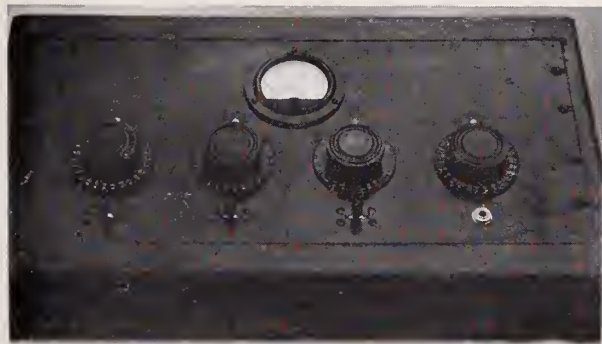
External Portable Mixer, Over All Gain and Volume Indicator Panel.
